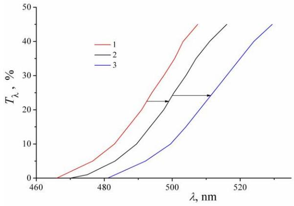
Fig. 3. Spectral transmission characteristics of as-prepared (1), annealed (2) and irradiated (3) TE a- $\text{As}_2\text{S}_3$  films
