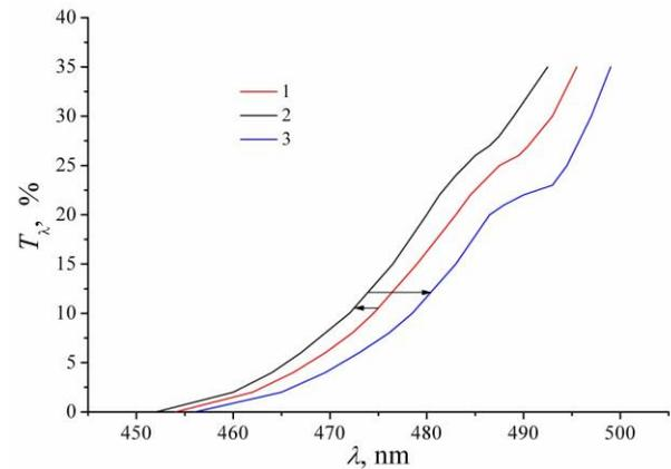
Fig. 4. Spectral transmission characteristics of as-prepared (1), annealed (2) and irradiated (3) RF a- $\text{As}_2\text{S}_3$  films
