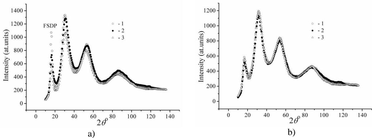
Fig. 5. X-ray diffraction intensity versus diffraction angle for TE- (a) and RF- (b) a-As<sub>2</sub>Se<sub>3</sub> films: 1- as-prepared, 2- annealed and 3-irradiated
