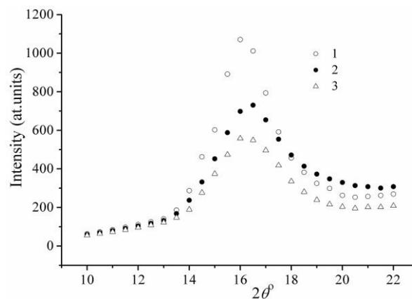
Figure 6. FSDP of as-prepared (1), annealed (2) and irradiated (3) TE a-As<sub>2</sub>Se<sub>3</sub> films
