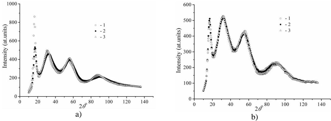
Figure 7. X-ray diffraction intensity versus diffraction angle for TE- (a) and RF- (b) a-As<sub>2</sub>S<sub>3</sub> films: 1 - as-prepared, 2 - annealed и 3 - irradiated
