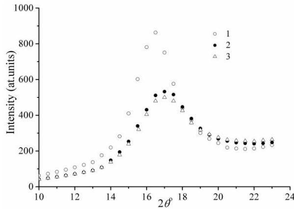
Figure 8. FSDP of as-prepared (1), annealed (2) and irradiated (3) TE a-As<sub>2</sub>S<sub>3</sub> films
