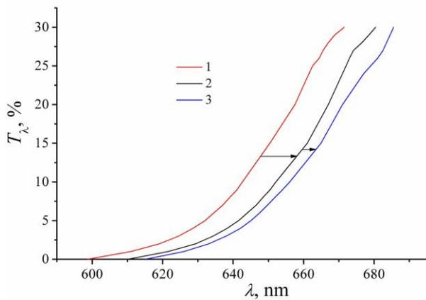
Fig. 1. Spectral transmission characteristics of as-prepared (1), annealed (2) and irradiated (3) TE a- $\text{As}_2\text{Se}_3$  films
