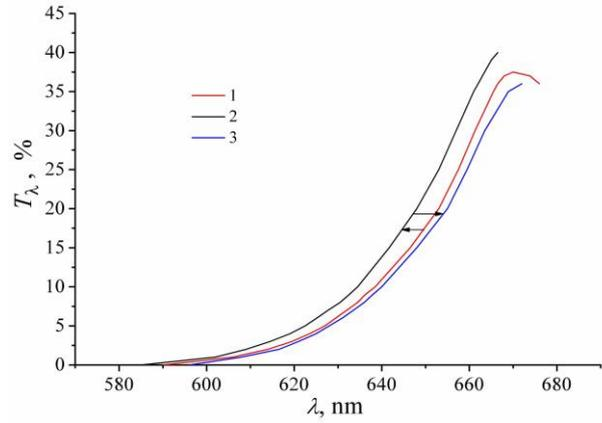
Fig. 2. Spectral transmission characteristics of as-prepared (1), annealed (2) and irradiated (3) RF a- $\text{As}_2\text{Se}_3$  films
