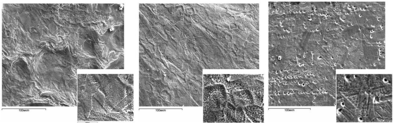
**Figure 2** - The surface of the samples № 1 ( $Q = 4,2 \text{ J/cm}^2$ ,  $n = 1$ ), № 3 ( $Q = 8 \text{ J/cm}^2$ ,  $n = 1$ ) and № 4 ( $Q = 22,8 \text{ J/cm}^2$ ,  $n = 1$ ) general view ( $\times 400$ ) and a fragment ( $\times 2000$ ) after treatment at  $P = 0.1 \text{ mm Hg}$
