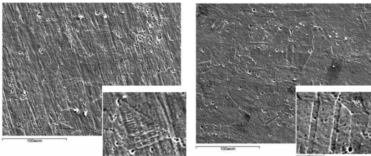
**Figure 3** – The surface of the sample number 2 ( $Q = 10,35 \text{ J/cm}^2$ ,  $n = 1$ ), № 3 ( $Q = 19,9 \text{ J/cm}^2$ ,  $n = 1$ ) general view ( $\times 400$ ) and a fragment ( $\times 2000$ ) after treatment with  $P = 0.5 \text{ mm Hg}$  respectively
