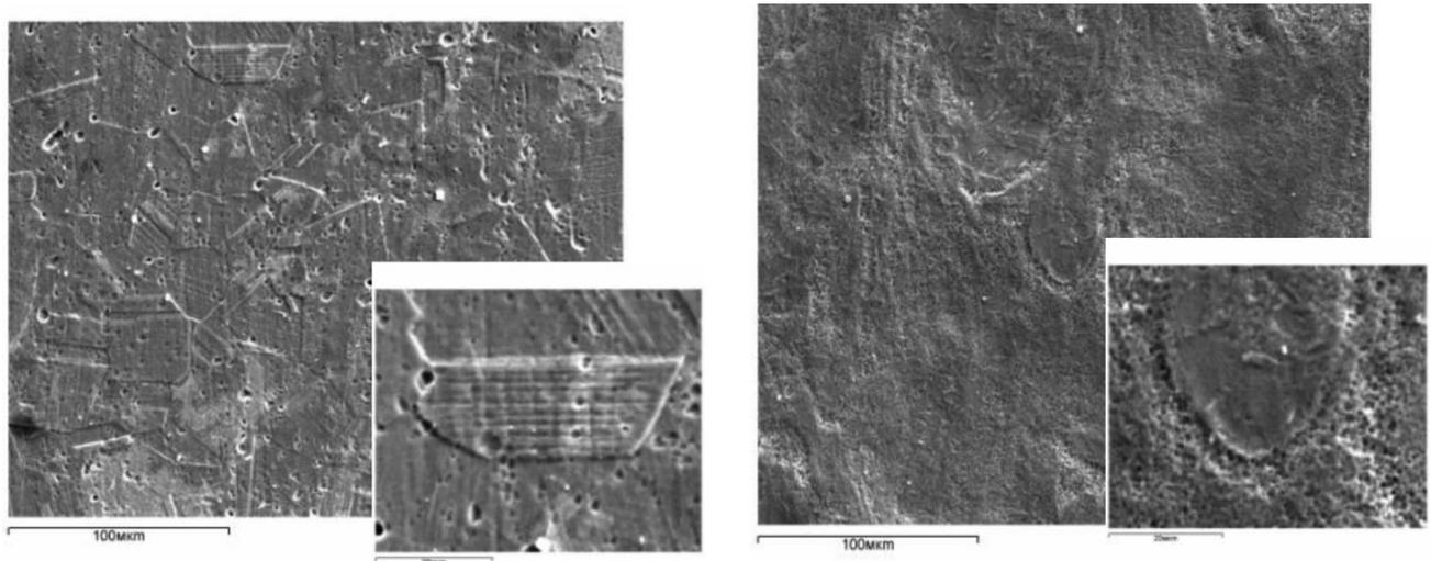
**Figure 1** – Topography of the sample number 1 ( $Q = 8,5 \text{ J/cm}^2$ ,  $n = 1$ ), № 4 ( $Q = 27,1 \text{ J/cm}^2$ ,  $n = 1$ ) general view ( $\times 400$ ) and a fragment ( $\times 2000$ ) after treatment with  $P = 0.04 \text{ mm Hg}$  respectively
