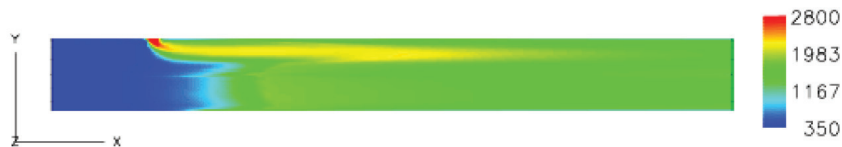
Figure 6 – Predicted temperature contours along the burner axial direction
