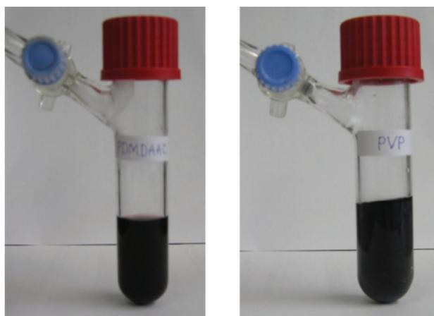
**Figure 1** – AuNPs stabilized by PVP and PDMDAAC
