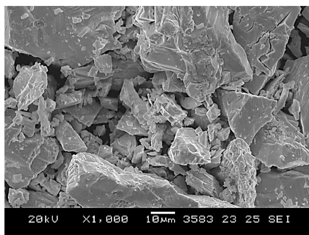
Figure 3 – SEM images of the starting holmium hydride powder at different magnifications
